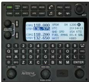
The optional ACD215 Control Panel provides easy access to all the FMS and radio tuning functions.
