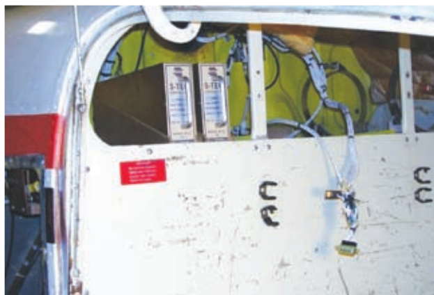
This Aztec equipment bay can accommodate extra remote boxes, but not all airframes will have room.
