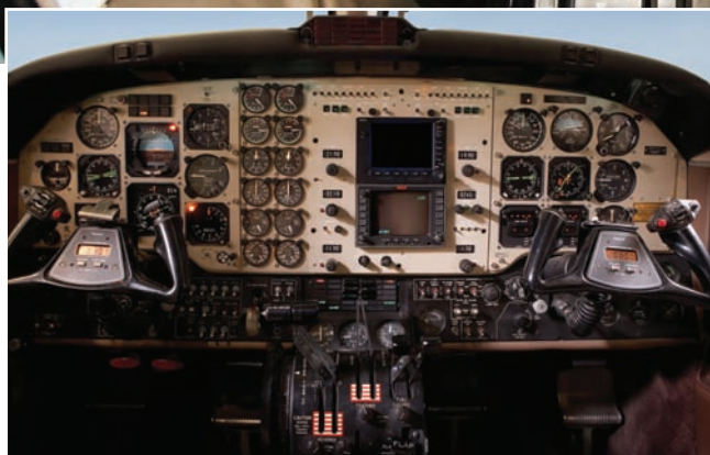
Compared to the original panel (left) the new Avidyne/S-Tec panel provides a plethora of new features for the King Air pilot, as well as an increase in useful load and greater situational awareness.
