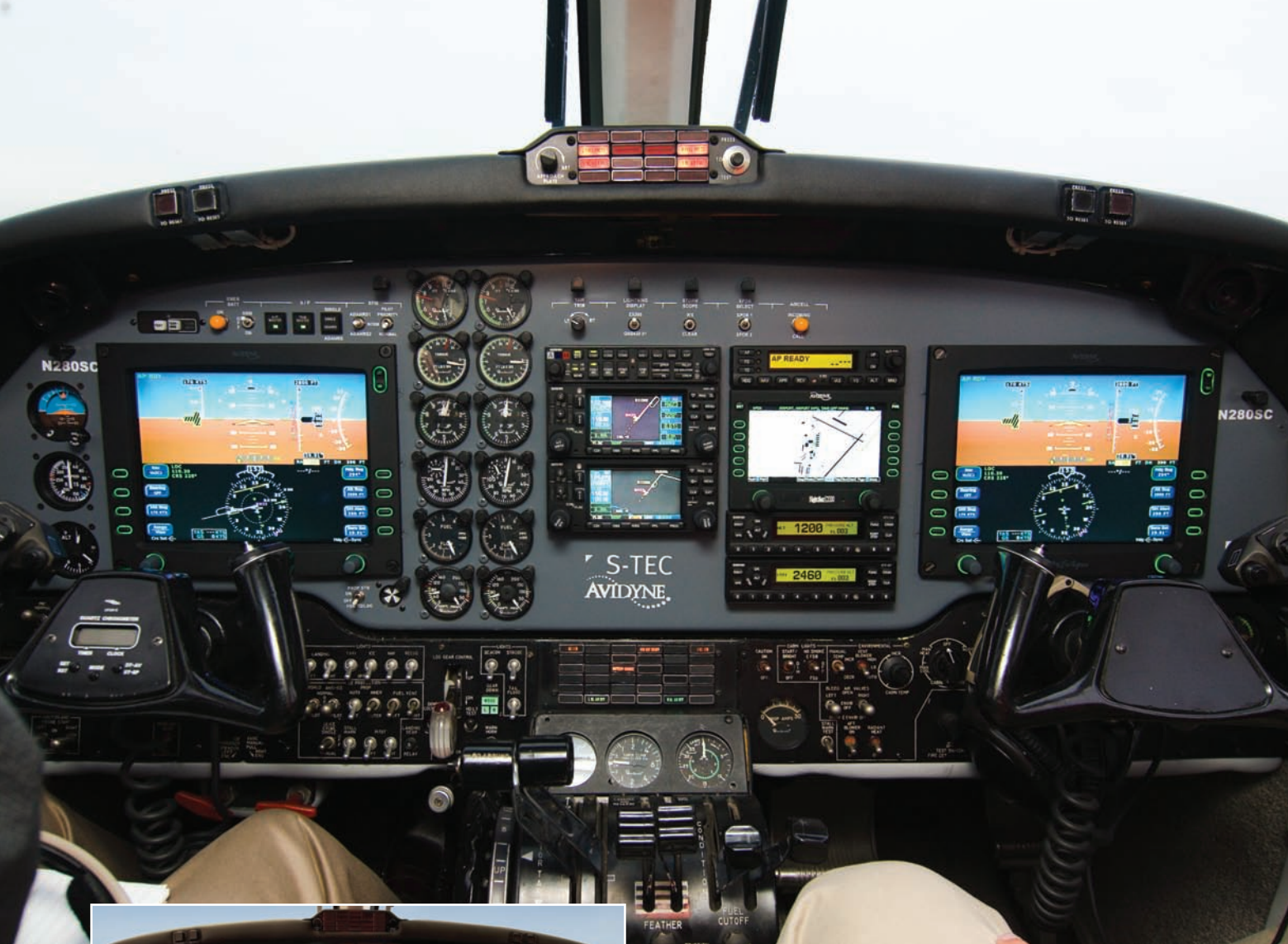
Compared to the original panel (left) the new Avidyne/S-Tec panel provides a plethora of new features for the King Air pilot, as well as an increase in useful load and greater situational awareness.
