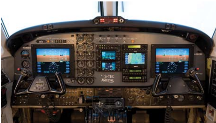
Alliant integrated flight deck from Avidyne and S-TEC.
