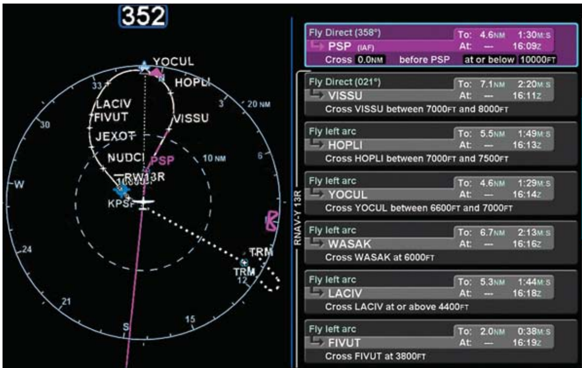
The map display clearly shows the path the FMS900w will guide the airplane over for an RNP arc approach to Palm Springs, including the possible missed approach path and holding. The flight plan information to the right of the map display describes each point in the procedure, including the crossing altitudes for the fix. Note the layout of the keys on the optional control display unit above.
