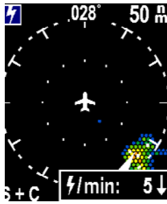
Figure 5.5 Five discharges per minute in the contiguous cell, and decreasing in rate. Blue dots indicate minimal activity.
