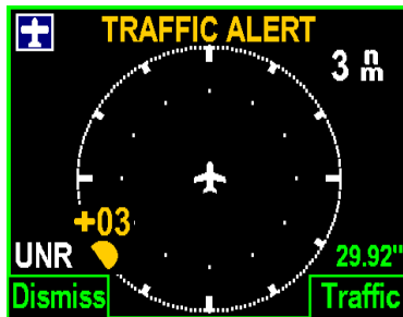
FIGURE 8.9 Special TA screen showing half a TA symbol for traffic that is beyond the three mile selected display range
