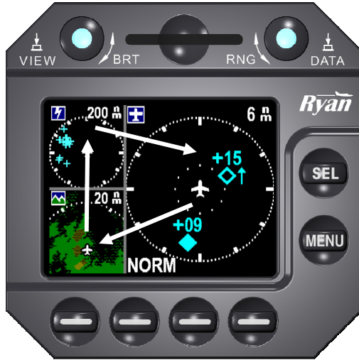
FIGURE 3.4 Multi-View Mode (the white arrows indicate the rotation sequence when SEL is pressed)
