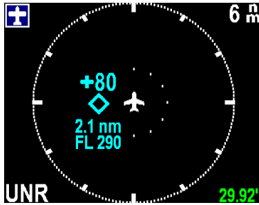
FIGURE 8.8 Extra data showing an OT intruder that is at flight level 290 (FL290)
