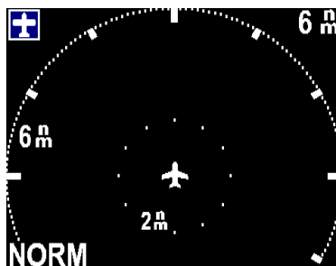
FIGURE 3.5 Example of the momentary duplicate range label shown while adjusting the range.
